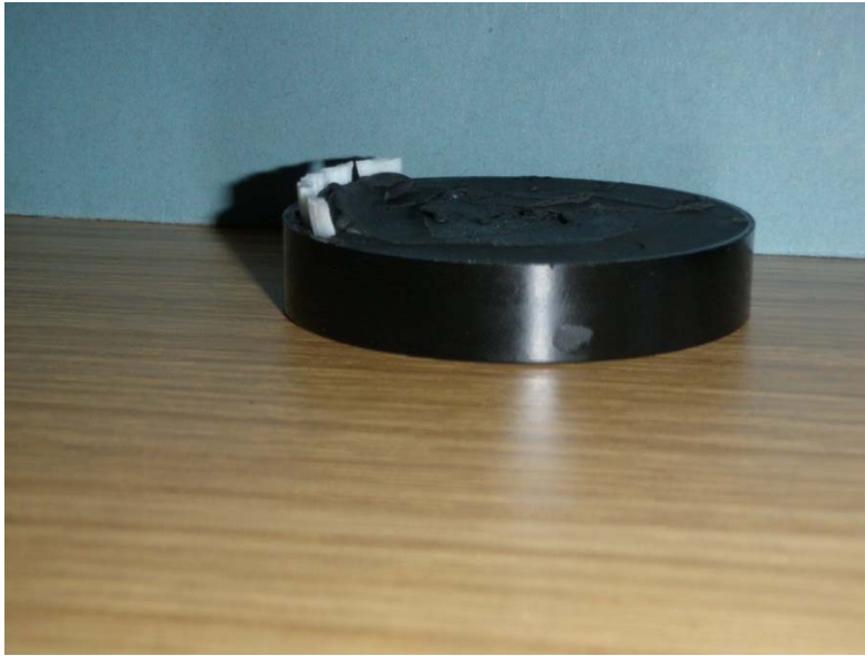
Figure 3. Mount with plasticine build up behind the otoliths.
