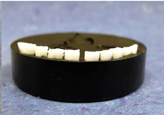
Figure 8. Side-view mounting in groups of five with a gap.
