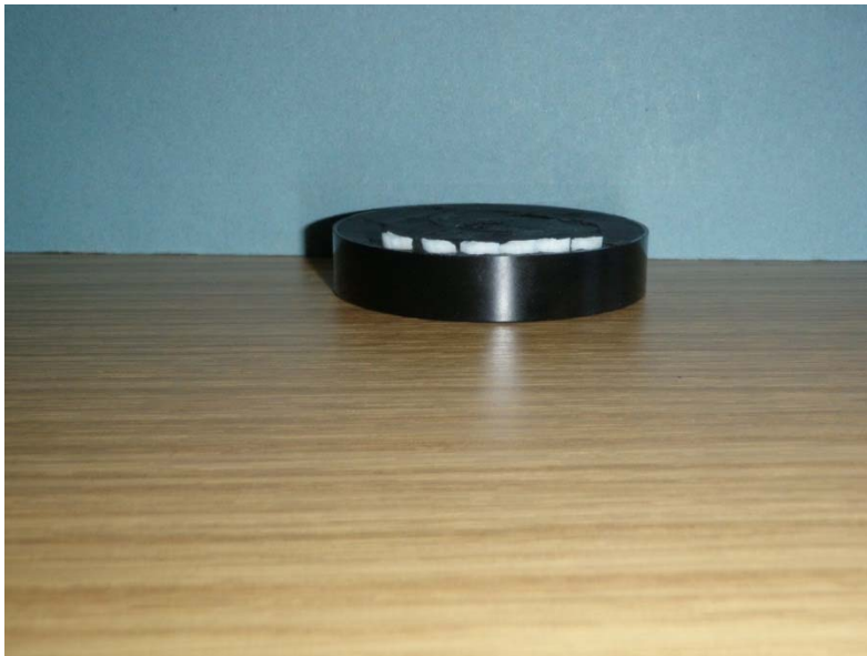
Figure 4. Mount showing otoliths too deeply embedded i.e. only 2mm showing
