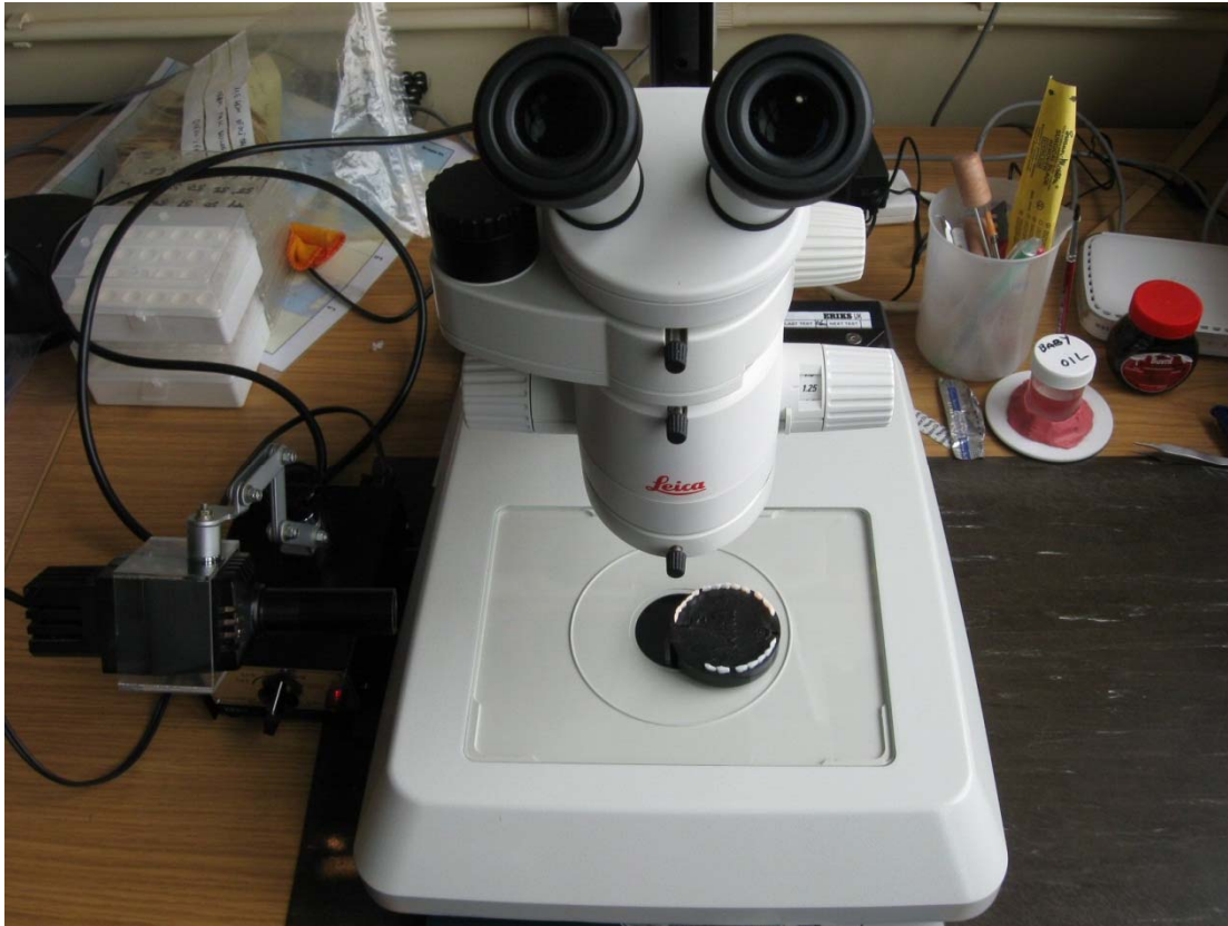
Figure 12. Photograph showing equipment setup used for age reading of gadoid otoliths (cod, haddock, whiting and saithe).
