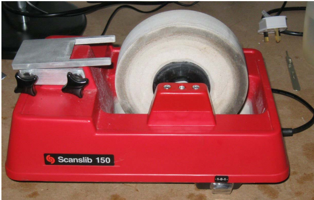
Figure 15. A wet stone grinder as used to grind flat the cut surface of otoliths which have not broken cleanly.
