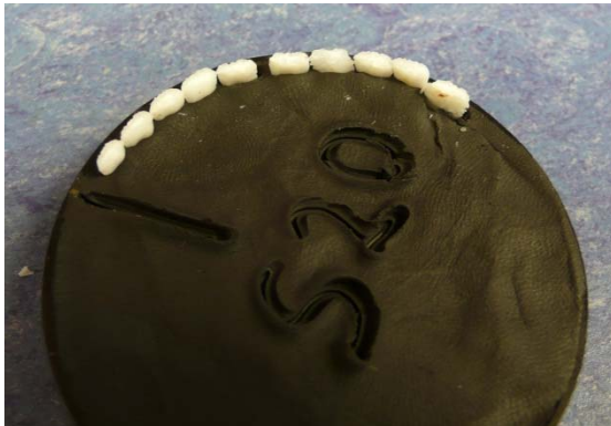
Figure 7. Top view of mounting in groups of five with a gap
