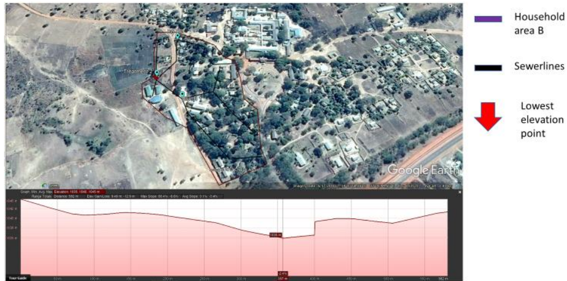
Figure 4-7: Sewer network 2 covering household area B
