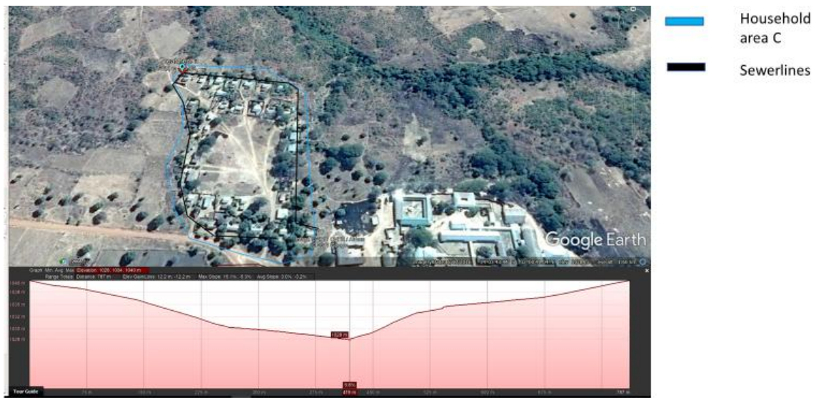
Figure 4-8: Sewer network 3 covering household area C
