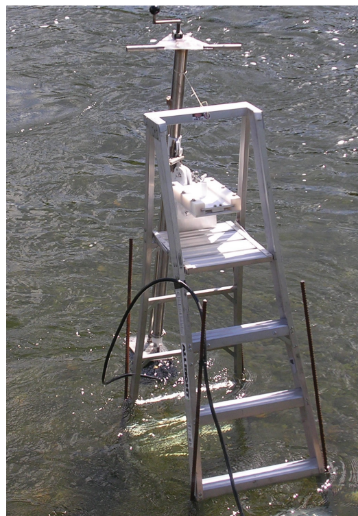
Figure 2.2. A simple stepladder mount for a DIDSON sensor. Photo courtesy of H. Enzenhofer.
