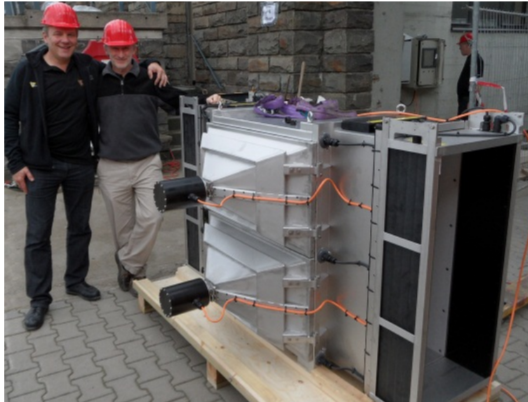
Figure 2.7. Vaki optical beam counter with double light box video recorder. Photo courtesy of Vaki.
