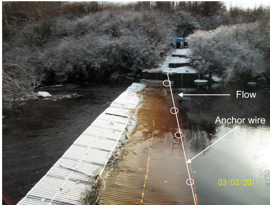
Figure 2.12. Keogh River Alaskan floating fence with 3 m long panels and trap box located on the far riverbank. Photo courtesy of InStream Fisheries Research.
