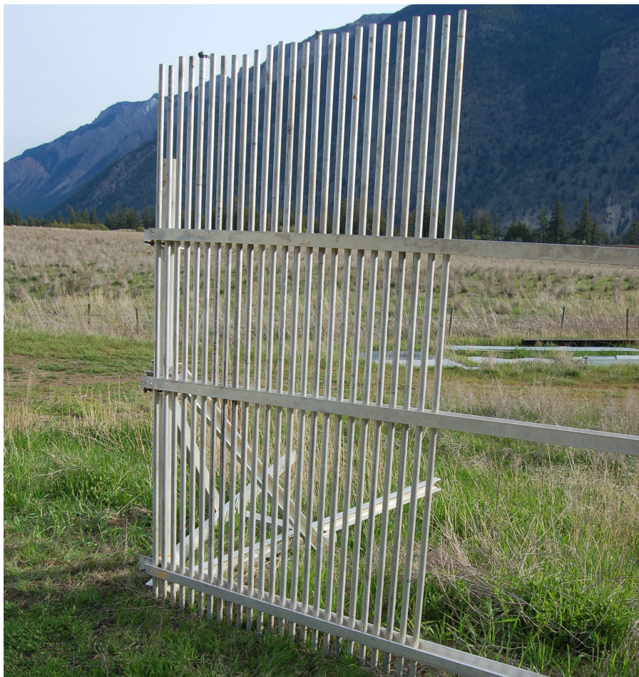
Figure 2.10. A single panel 10 ft high picket fence with mounting tripod and three rails. Photo courtesy of InStream Fisheries Research.
