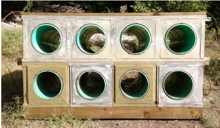
Figure 2.20. Seton Dam fish pass sensor units prior to installation in a separation grid. Photo courtesy of InStream Fisheries Research.
