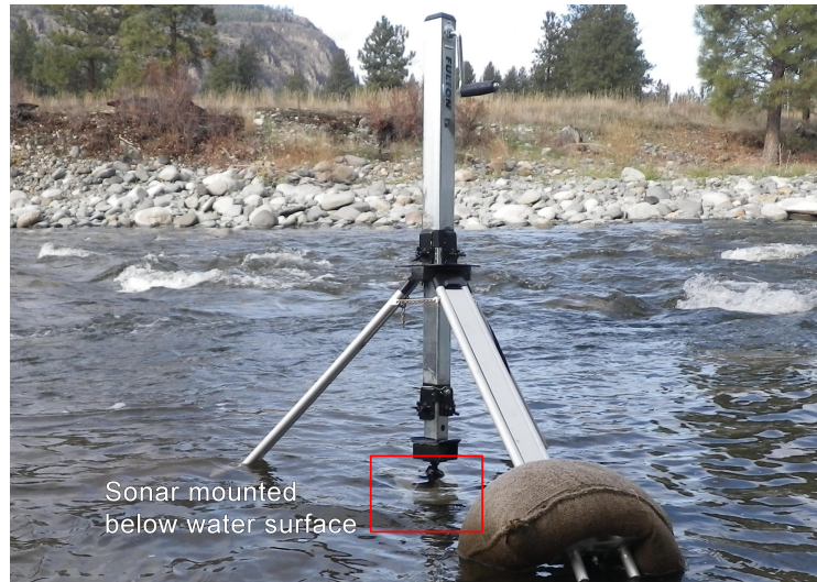
Figure 2.1. Sonar unit mounted on the bottom of a tripod at Spius Creek, held to the substrate by sandbags. This installation allows adjustment with a winch above water surface. Photo courtesy of H. Olynyk – DFO.
