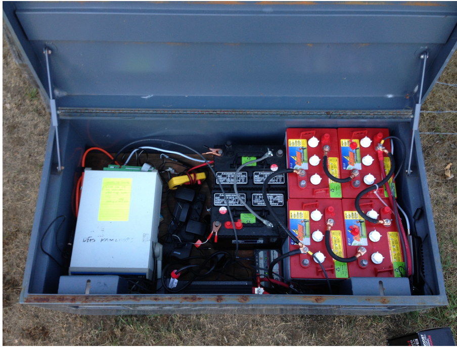
Figure 2.3. Logie resistivity counter setup with battery bank. Photo courtesy of InStream Fisheries Research.
