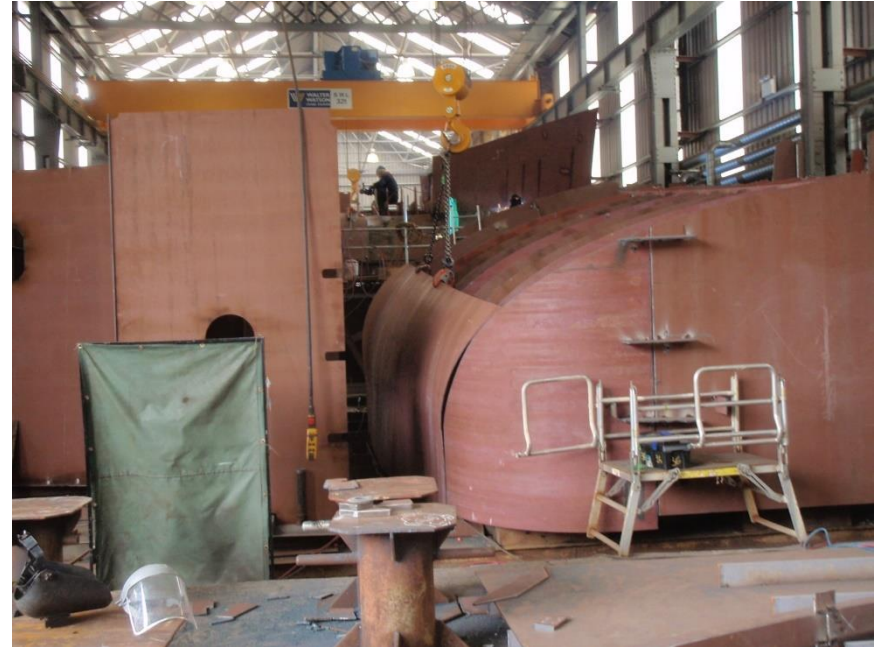
Vessel 1 – Stern Units Under Construction
