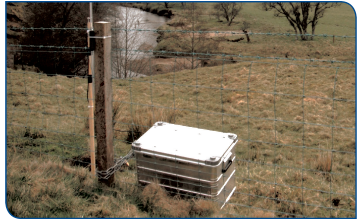
FIGURE 2 A RECEIVER STATION ON THE SOUTH ESK, EACH FISH IS FITTED WITH A MINATURE RADIO TRANSMITTER (SEE BELOW)
