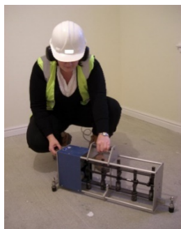
Figure 4 Impact sound test being carried out
